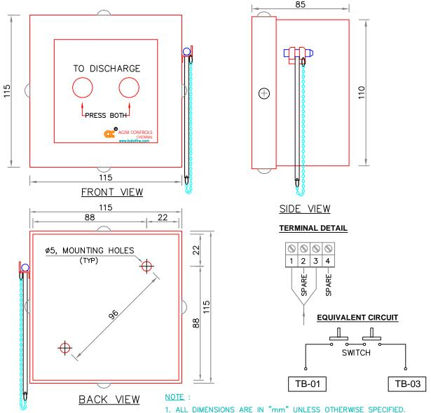
2. TOLERANCE ON DIMENSION  $\pm$  3 MM, UNLESS OTHERWISE SPECIFIED.
